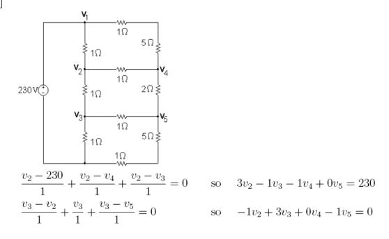
$$\frac{v_4 - v_2}{1} + \frac{v_4 - 230}{6} + \frac{v_4 - v_5}{2} = 0 \qquad \text{so} \qquad -12v_2 + 0v_3 + 20v_4 - 6v_5 = 460$$
